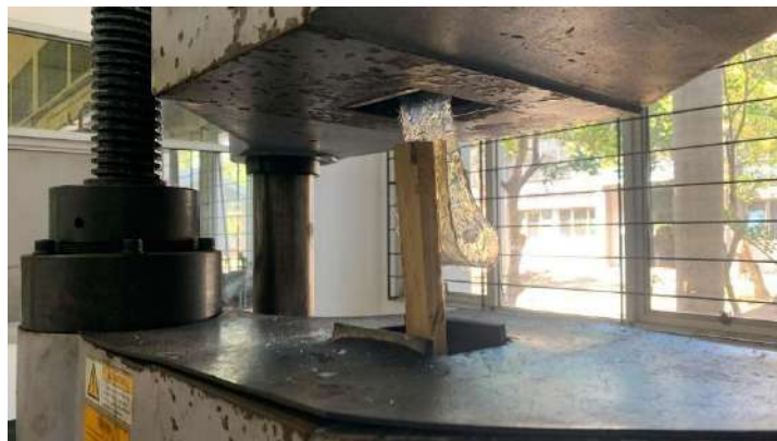
Gambar 4.11 Proses peel test variasi laminasi epoxy
