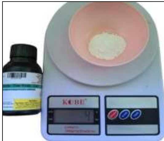
Gambar 3. 5 Takaran Active Flux \text{ZnO}
