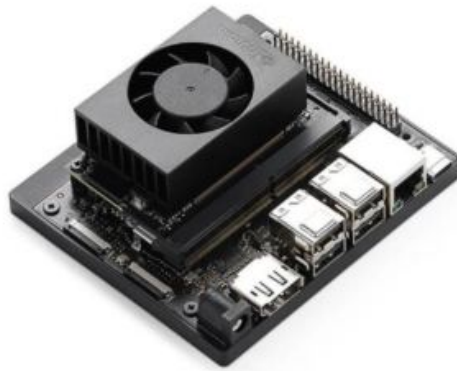
Gambar 2. 11 NVIDIA Jetson Orin Nano (Sumber: alibaba.com)
