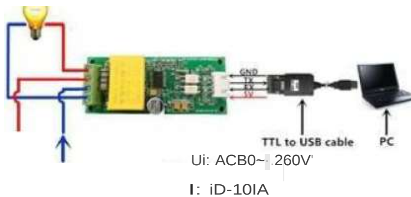
Figure 4.1: PZEM-004T-10A module wiring diagram
