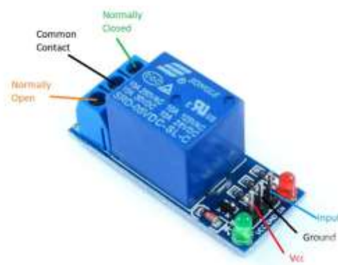
Gambar 2.9 Relay 5V
