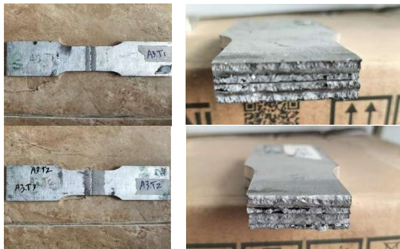
Gambar 4. 28 Hasil Patahan Uji Tarik Filler 5356 110° (A3)
