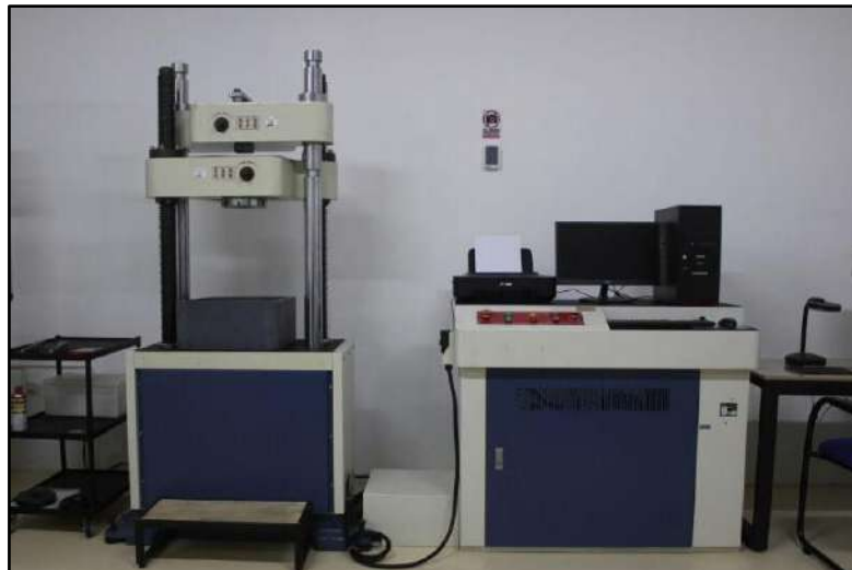
Gambar 2. 16 Mesin Uji Tarik (Munir, 2019)
