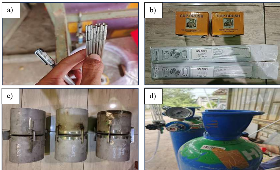
Gambar 3. 3 a). Filler Metal ER308L, b). Elektroda E308-16, c). Spesimen Stainless Steel SA-312 TP304, dan d). Argon High Purity 99,98%
