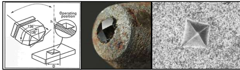
Gambar 2. 17 Prinsip Uji Vickers (Munir, 2019)
