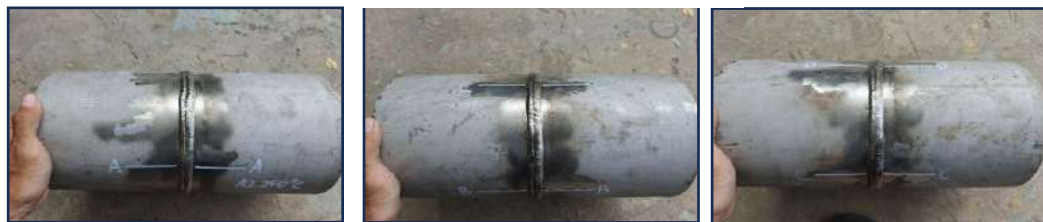
b). Interpass Temperature 250 °C
