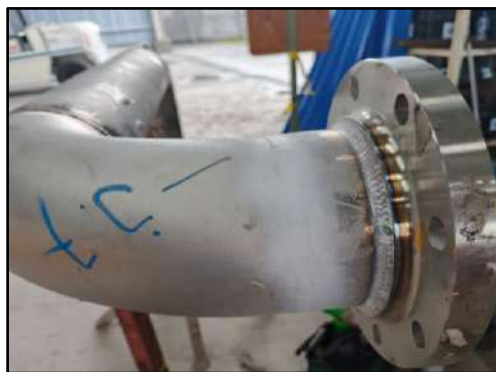
Gambar 2. 2 Produk Pipa Stainless Steel SA-312 TP304
