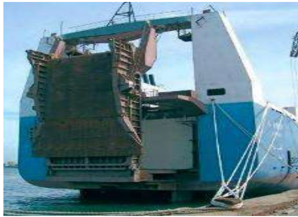
Gambar 2. 4 Slewing Ramp Door ( www.macgregor.com )
