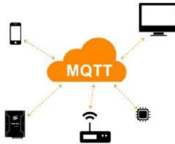
Gambar 2.25 Topologi Protokol MQTT (Sumber : https://iotstudio.labs.telkomuniversity.ac.id/ )
