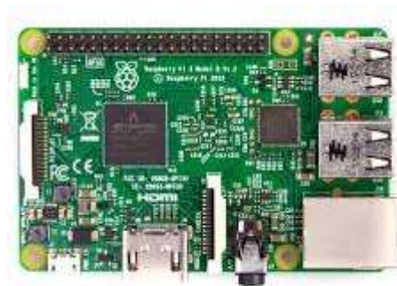
Gambar 2.13 Raspberry pi 3 Sumber: https://l1nq.com/elnayuj
