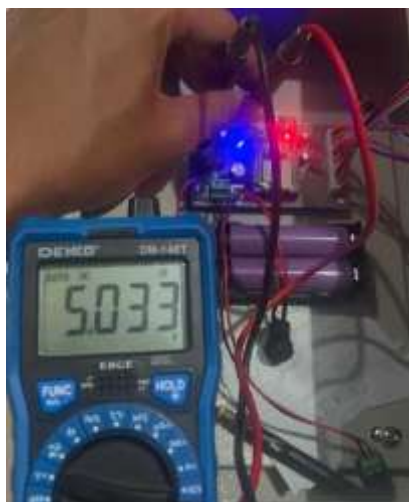
Gambar 4.4 Pengujian Parsial Output Buck Converter
