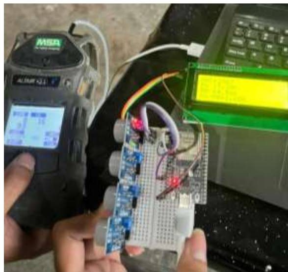
Gambar 4.5 Pengujian Parsial Sensor MQ-7
