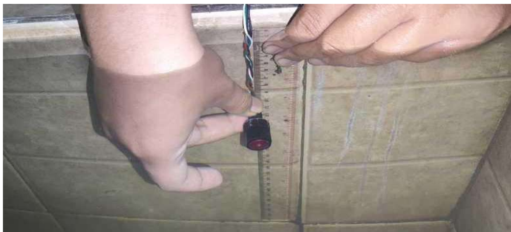
Gambar 4. 4 Pengujian Sensor Pressure MS5837
