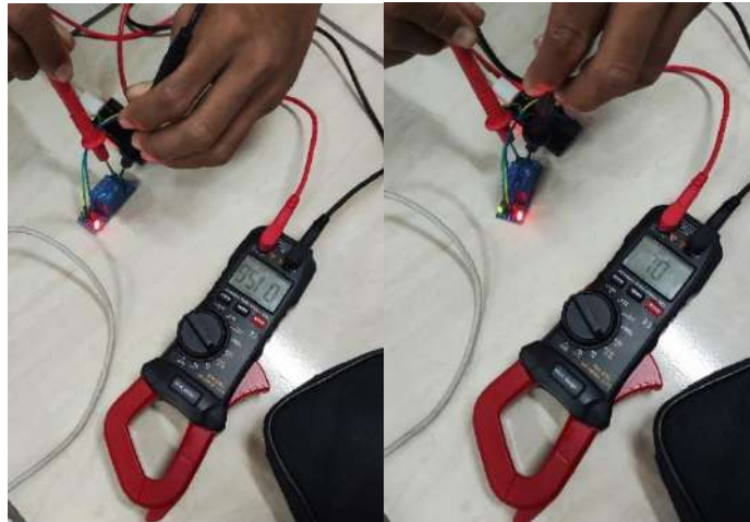
Gambar 4. 20 Pengujian Relay 5V 1 Channel
