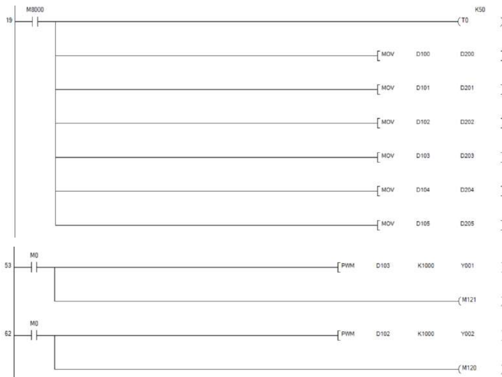
Gambar 3. 13 Function Block PWM GX Works2
