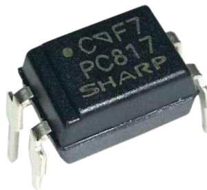
Gambar 2. 13 Optocoupler PC817 (Sumber: Tokopedia)
