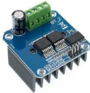
Gambar 2. 12 Driver BTS7960 (Sumber: Athoillah et al, 2021)
