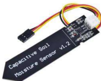
Gambar 2. 8 Sensor Moisture Kapasitif (Sumber: Taryana, 2021)
