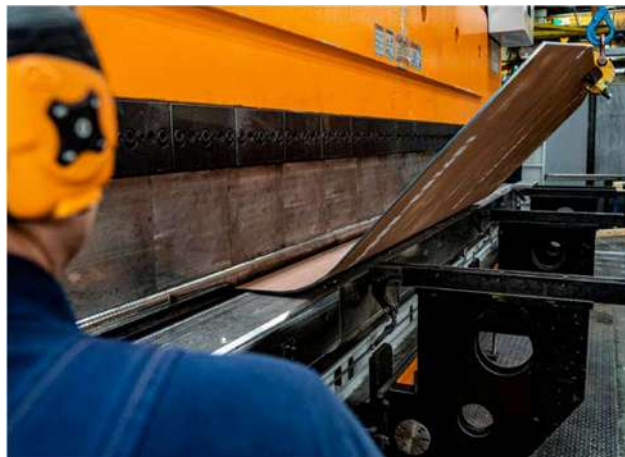
Gambar 2. 4 Proses cold bending (SSAB, 2023)
