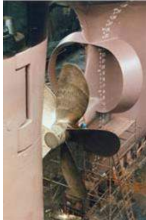
Gambar 2.5 Wake Equalizing Duct (WED)
