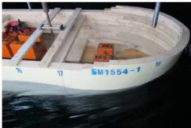
Photo 6 Bow Wave Pattern [11kn, Design Draught]
