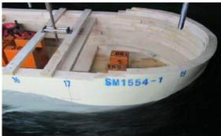
Photo 8 Bow Wave Pattern [12.5kn, Design Draught]
