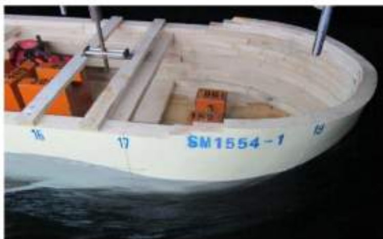
Photo 7 Bow Wave Pattern [12kn, Design Draught]
