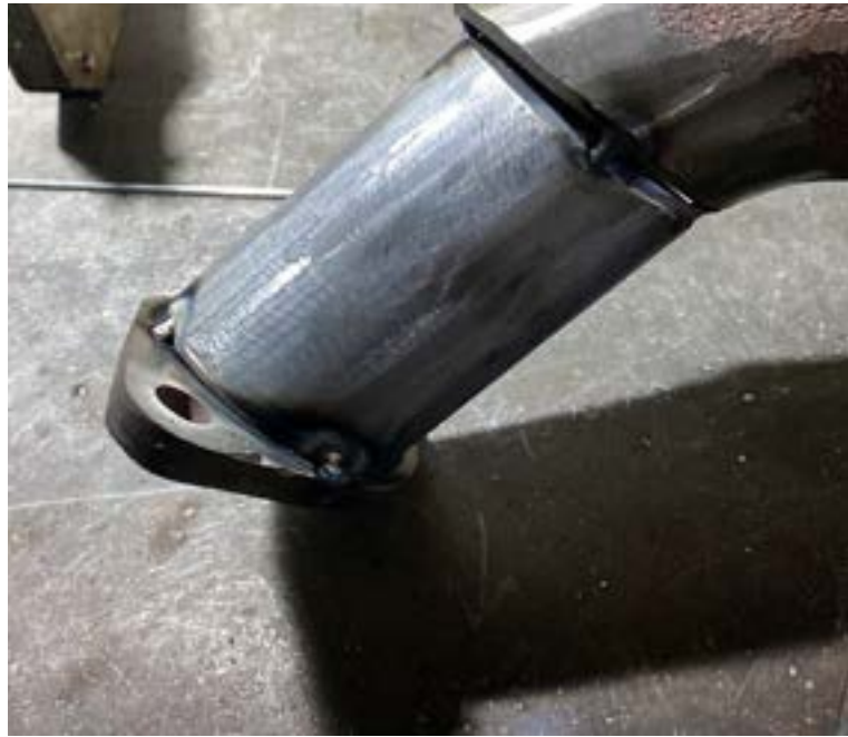
Gambar 4. 4 Proses pengelasan Intake manifold 52 cm
