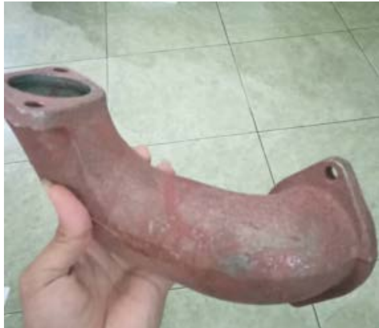
Gambar 4. 1 Intake manifold standart 32 cm
