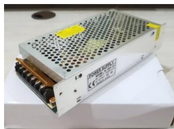
Gambar 2.14 Power supply 12 volt (Sumber: orbit.co.id )
