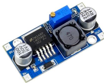
Gambar 2.13 Buck Converter (Sumber : addicore.com)
