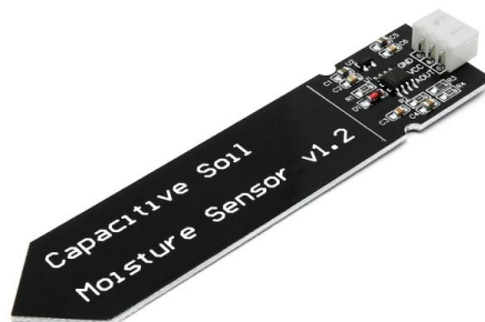
Gambar 2.7 Sensor Capacitive Soil Moisture (Sumber: thepihut.com)
