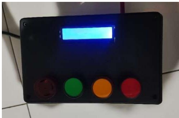
Gambar 4. 14 Keadaan aktual lampu saat relay OFF
