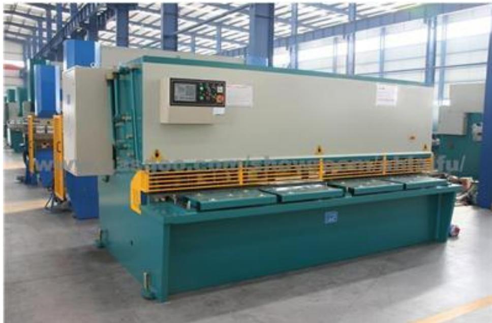
Gambar 1.2 Hydraulic Cutting Machine
