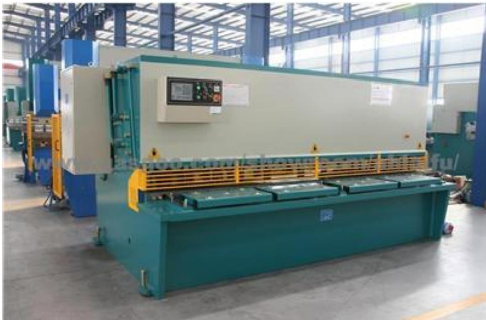
Gambar 1.2 Hydraulic Cutting Machine
