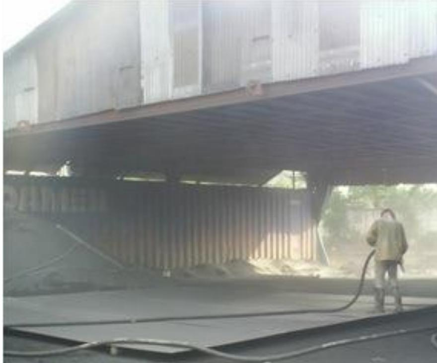
**Gambar 1.4** Proses Sand Blasting
