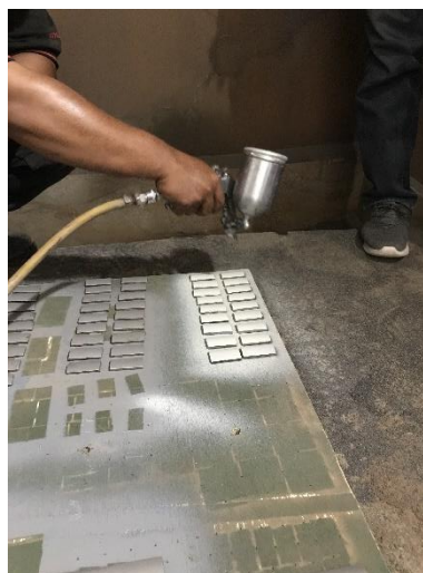
Gambar 4.10 Proses painting menggunakan conventional spray
