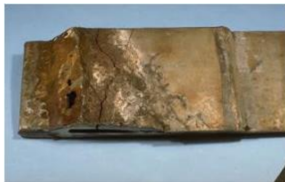
Gambar 2.7 Stress Corrosion Cracking
