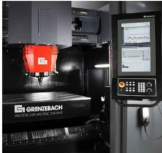
Gambar 2.4 Controller FSW ( Friction Welding Handbook , .2017)
