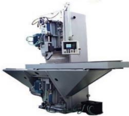
Gambar 2.1 Mesin Friction Stir Welding ( Friction Welding Handbook ESAB, 2019)
