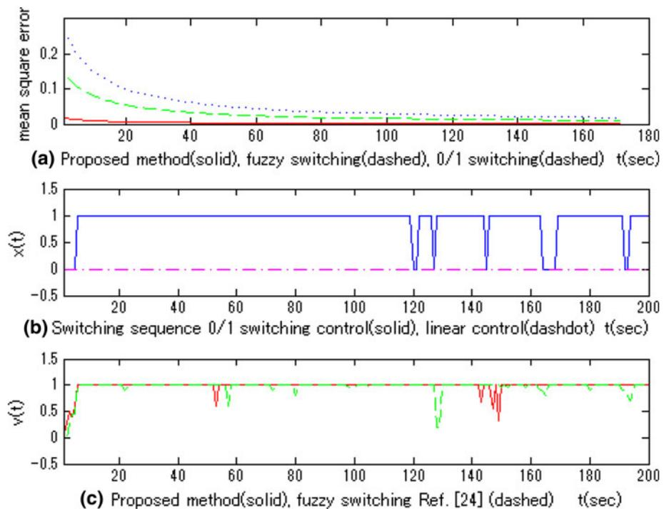
last half time. In Fig. 1c, the green dashed line shows the fuzzy switching control output  $y_2(t)$ . From the figure, it is shown that the proposed control method can do better than fuzzy switching controller.
