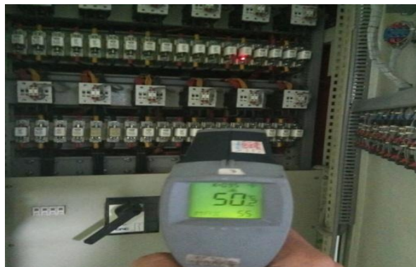
Gambar 2.2 pengukuran suhu panel mdp no 06
